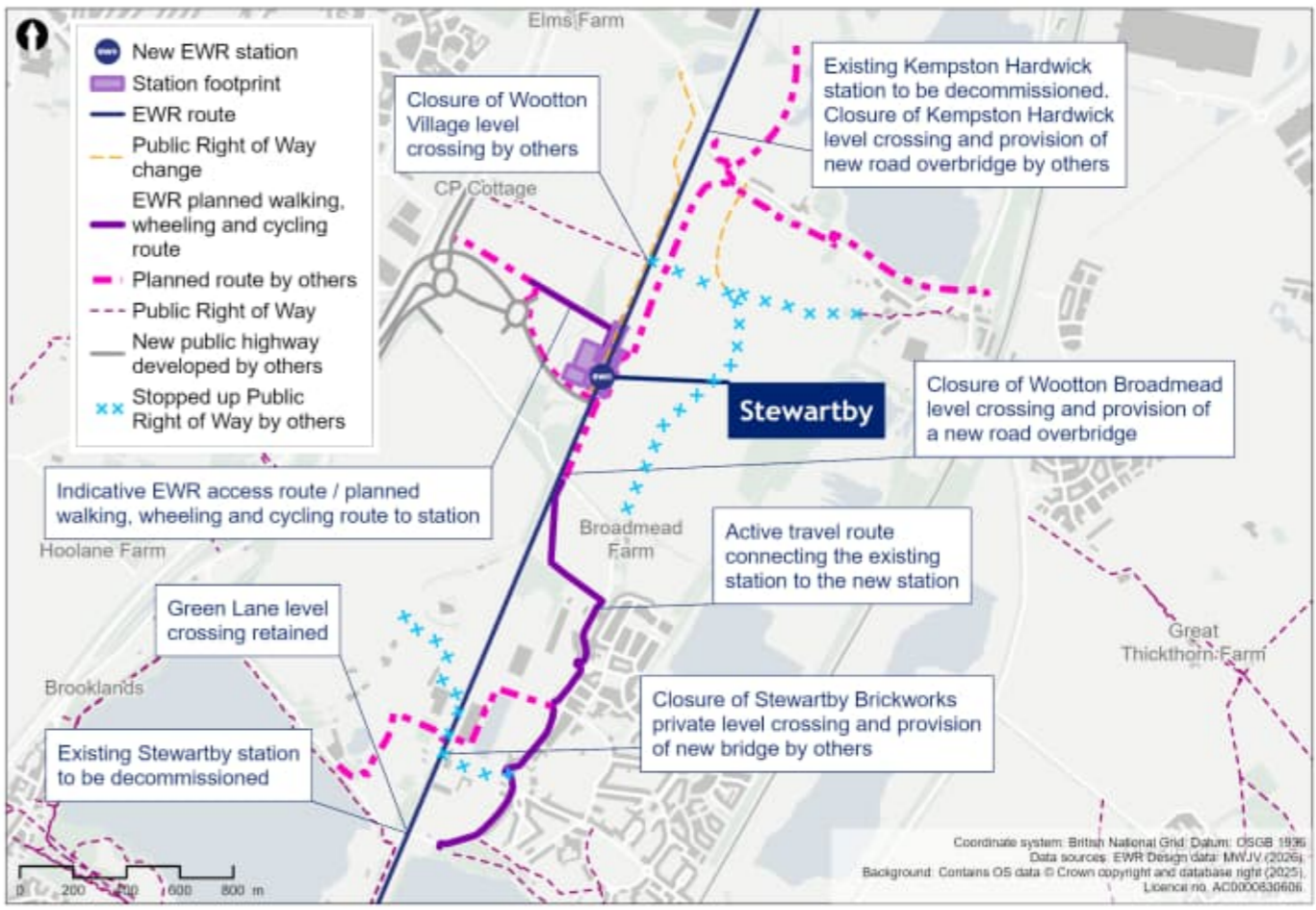
Figure 47: Map showing our proposals for level crossings around the new Stewartby station
